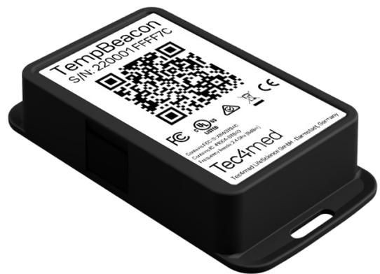
The TempBeacon serves as an intelligent temperature and humidity data logger with advanced capabilities. It effectively records all data internally and offers two methods of data retrieval: manual access through the Tec4App and automated retrieval via the SmartHub gateway.
